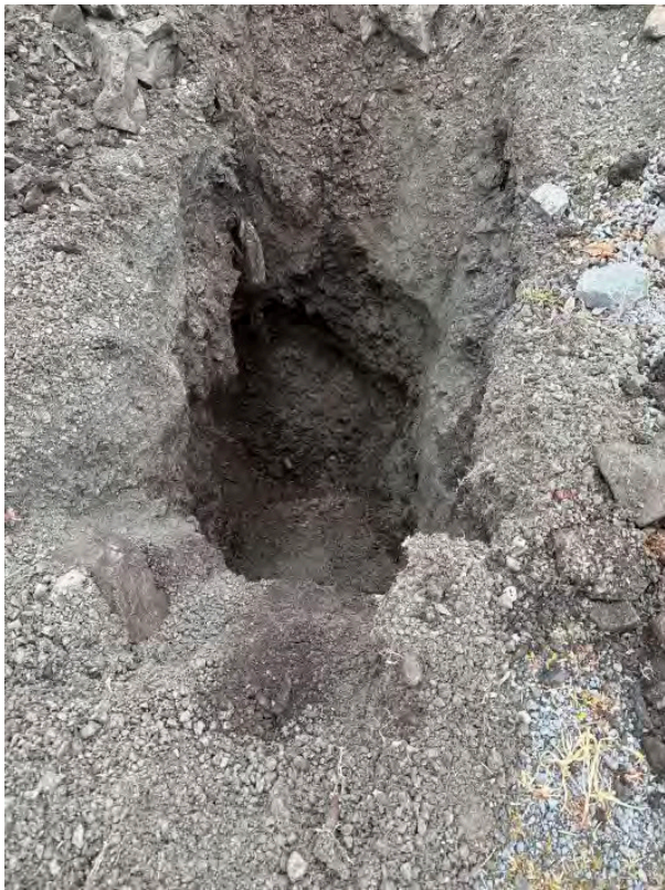
Unit 5. SW 208°. Mix of road fill on the south side of the excavation and natural material on the north at 9 feet below the surface where excavation testing was halted.
